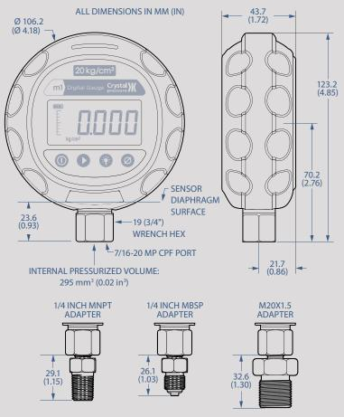
ADDITIONAL SENSOR LENGTH WITH OPTIONAL FITTING ADAPTERS
